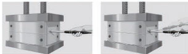
Surface temperature measurement of mold
