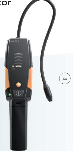
testo 316-3 is a reliable leakage detector for refrigerants which should be a part of every professional's refrigeration technology equipment. It detects even the smallest leaks thanks to its high level of sensitivity of 4 g/a, and fulfils the requirements of the F-gas regulation as well as the standards SAE J1627 and EN14624:2012.
